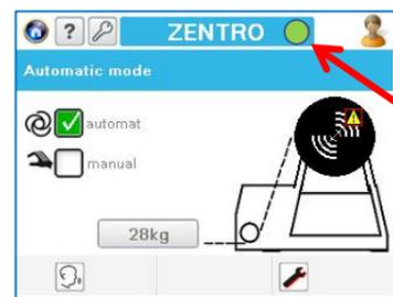
Supervision of running signal 'weaving machine' and connection check.
